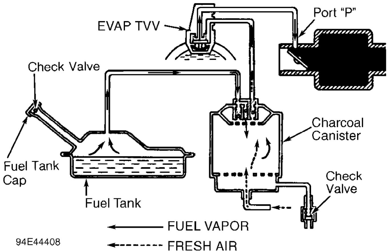
Fig. 6: Identifying Typical EVAP System Components
