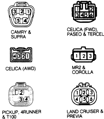
Fig. 1: Fuel Sending Unit Harness Connector Terminal ID Courtesy of Toyota Motor Sales, U.S.A., Inc.
