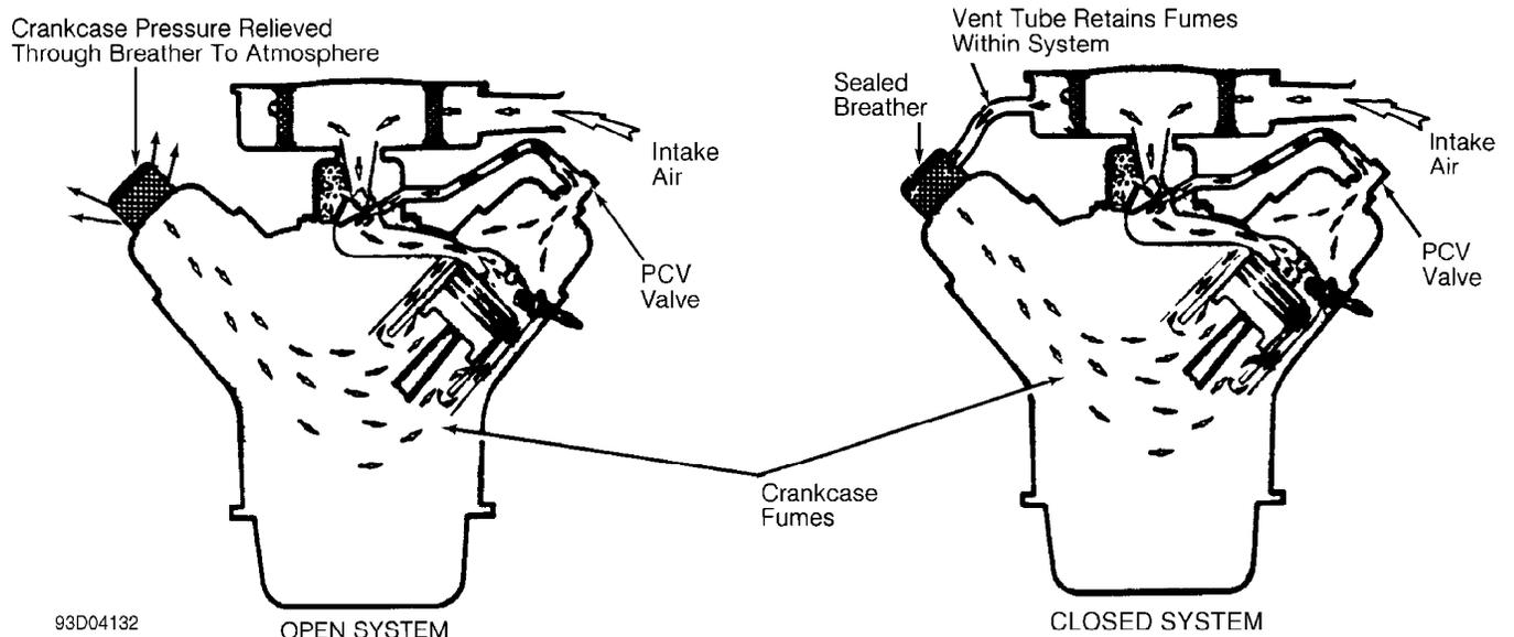
Fig. 2: Typical Open & Closed Type PCV System
