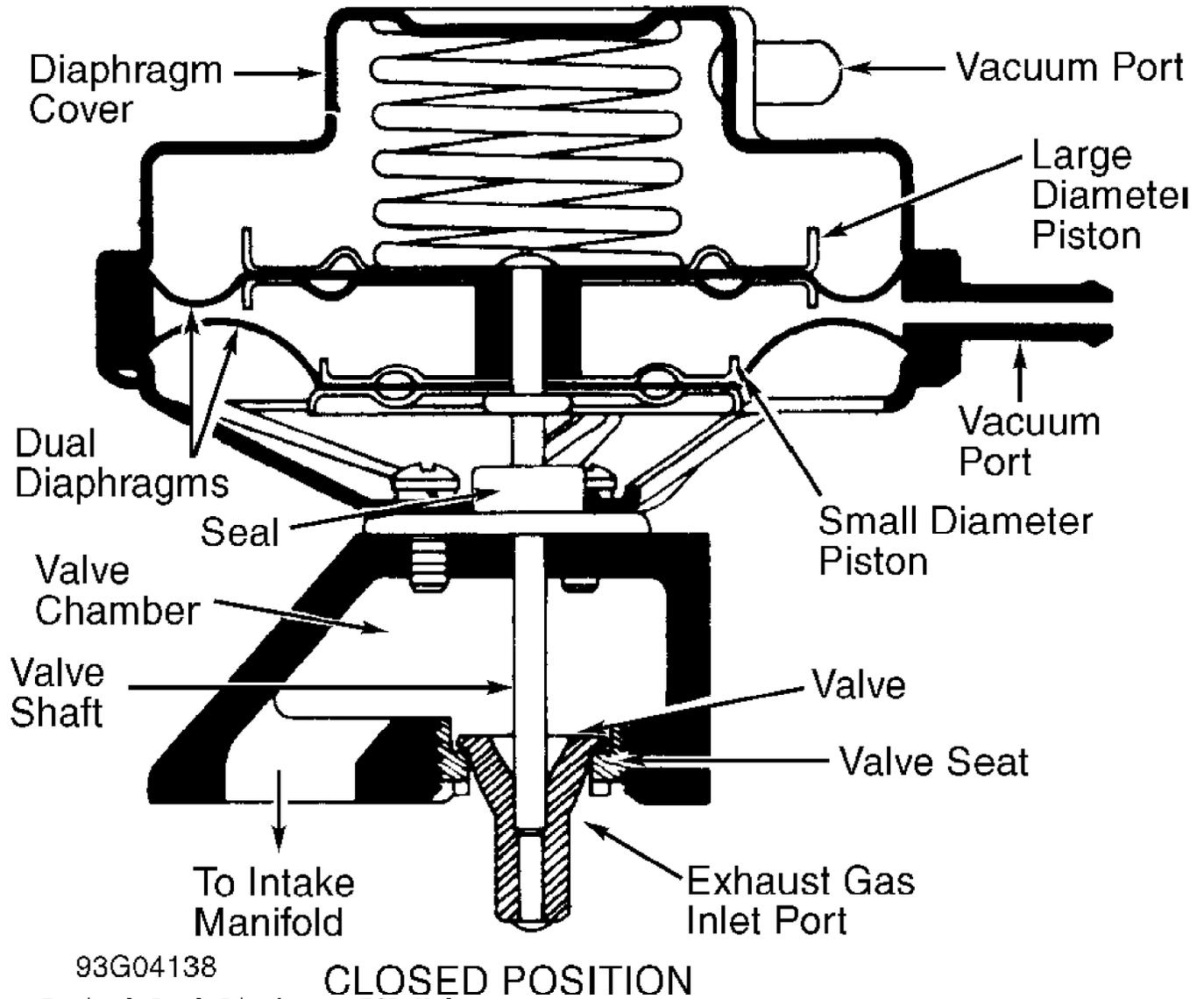
Fig. 8: Typical Dual Diaphragm EGR Valve
