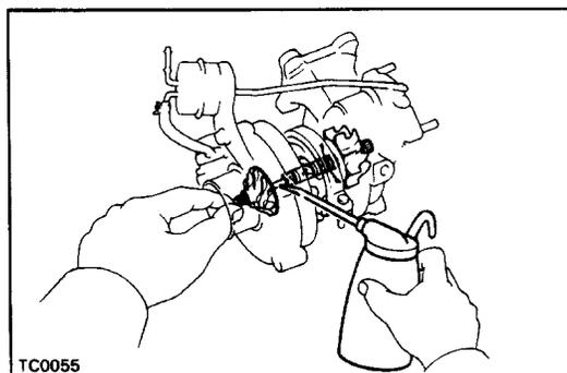
5. Use caution when removing and reinstalling the turbocharger assembly. Do not drop it or bang it against anything or grasp it by easily-deformed parts, such as the actuator or rod, when moving it.
