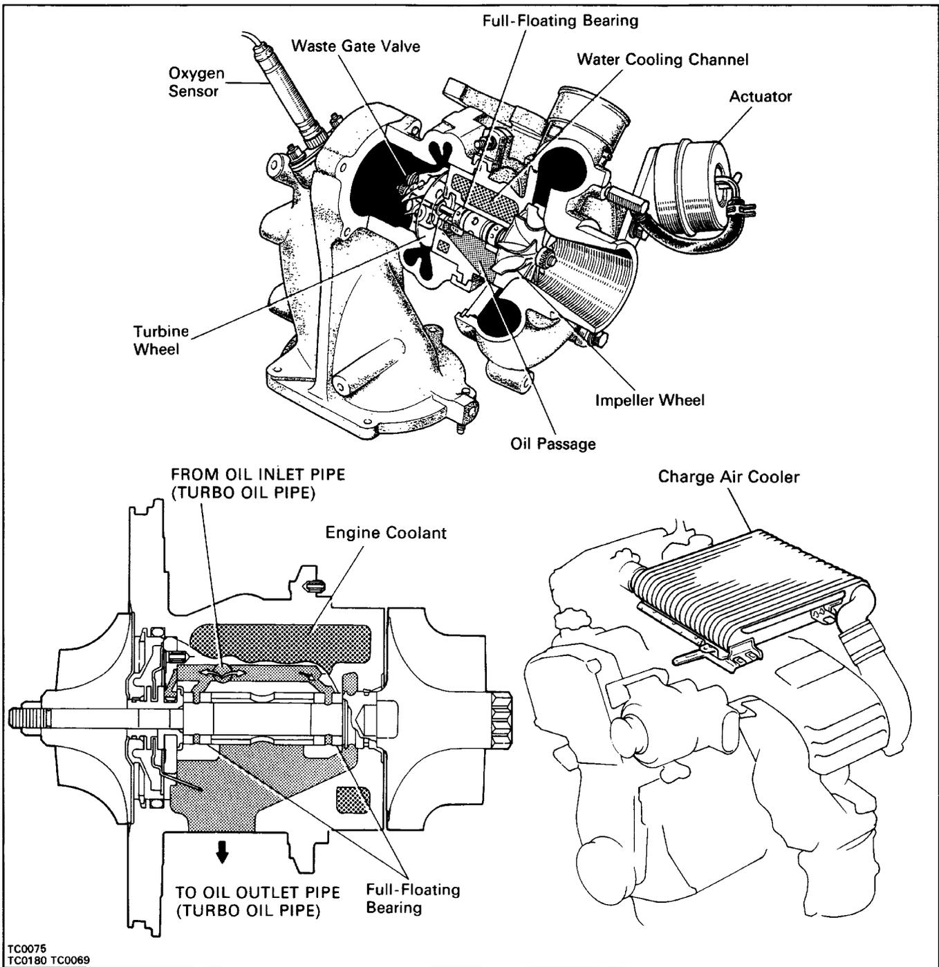
Systems which increase the amount of air sent to the engine are either turbocharger type (using exhaust gas to turn the turbine) or supercharger type (using the engine crankshaft, etc. to mechanically turn the pump, etc.). For CELICA 3S-GTE engine, the turbocharger type has been adopted.
