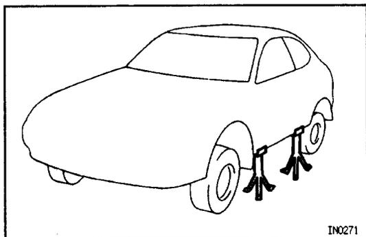
1. **JACK UP VEHICLE SO THAT ALL FOUR WHEELS CLEAR GROUND AND CAN BE ROTATED**
