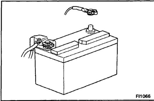
1. Malfunction symptoms of the airbag system are difficult to confirm, so the diagnostic codes become the most important source of information when troubleshooting. When troubleshooting the airbag system, always inspect the diagnostic codes before disconnecting the battery (See page [AB-24](#)).
