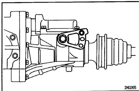
**6. AFTER FINISHING TEST, RETURN MODE SELECT LEVER TO "VISCOUS (NORMAL) MODE" POSITION AND INSTALL SET BOLT**
