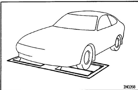
1. MOVE MODE SELECT LEVER ON TRANSAXLE TO "VISCIOUS FREE MODE" AND INSTALL SET BOLT (See page IN-15)
