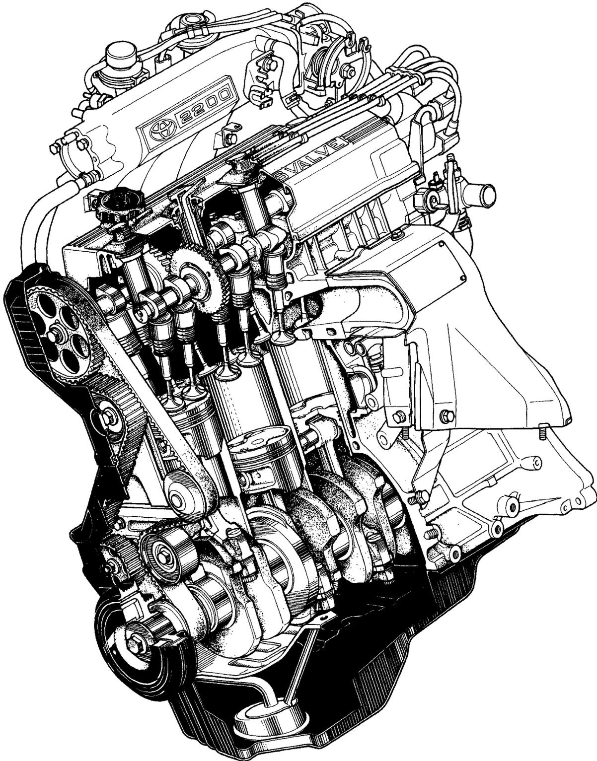
The 5S-FE engine is an in-line, 4-cylinder engine with the cylinders numbered 1 – 2 – 3 – 4 from the front. The crankshaft is supported by 5 bearings inside the crankcase. These bearings are made of aluminum alloy.
