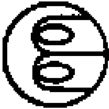
Fig. 15: Internal Fuse, Thermal Limiter
