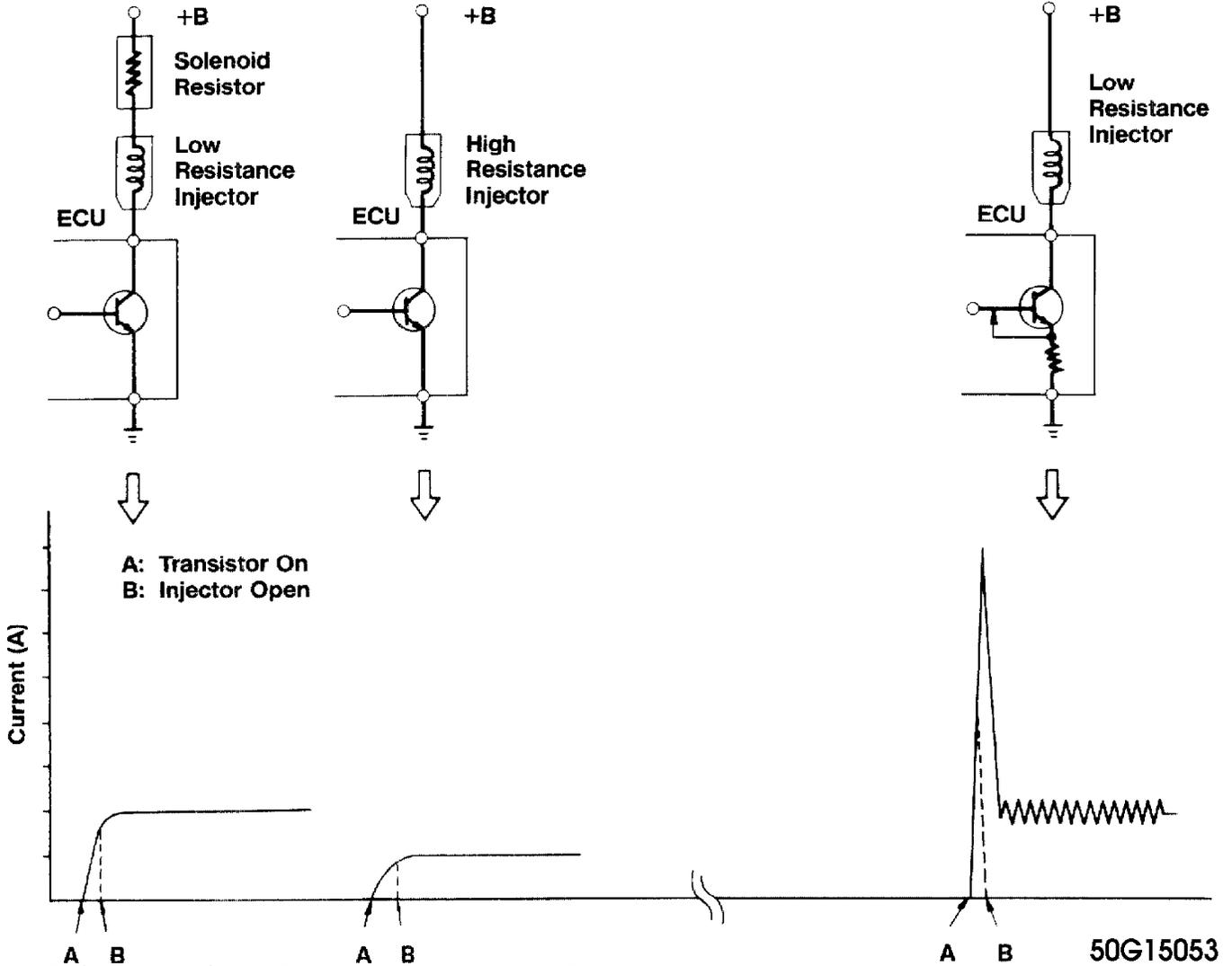
Fig. 1: Injector Driver Types - Current and Voltage
