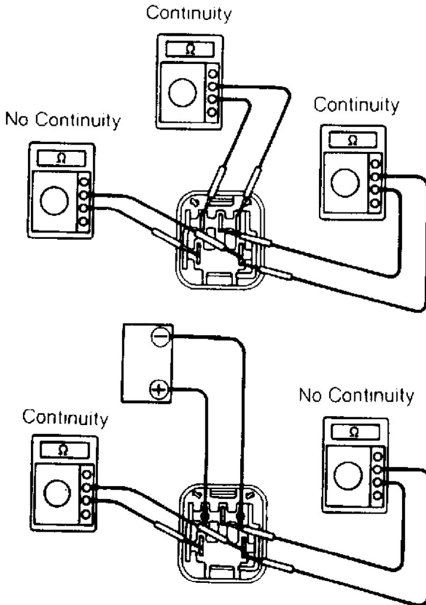
Fig. 9: Testing Engine Main Relay
