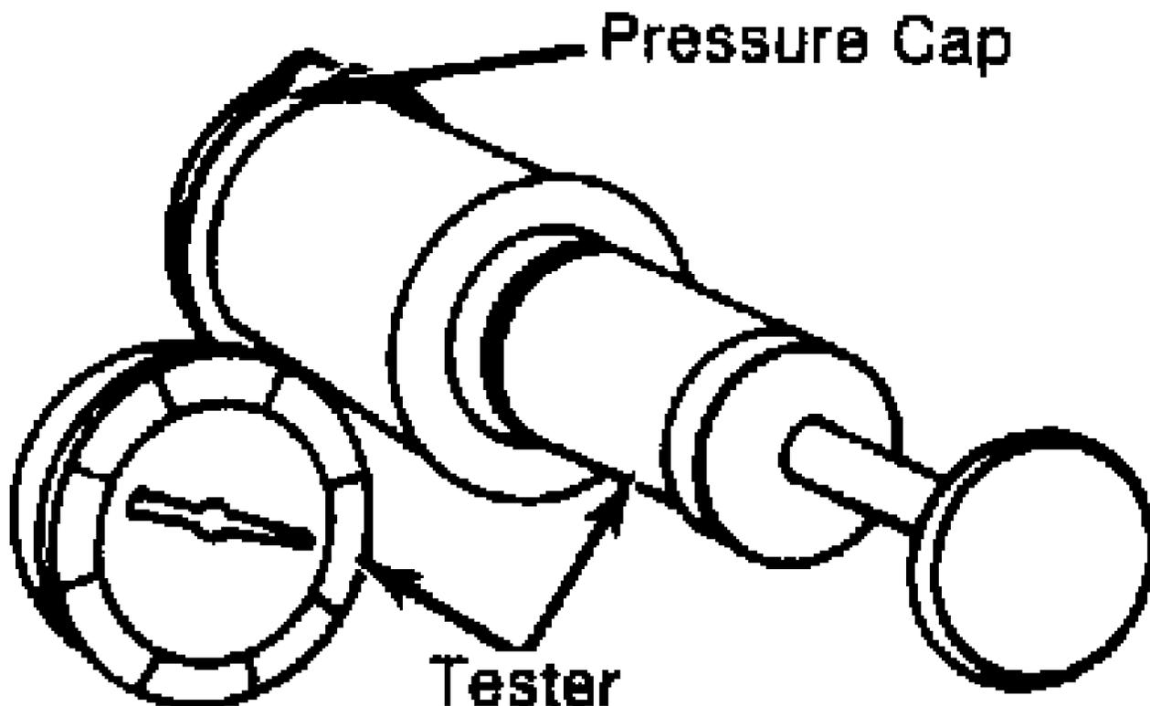
Fig. 2: Testing Radiator Pressure Cap
