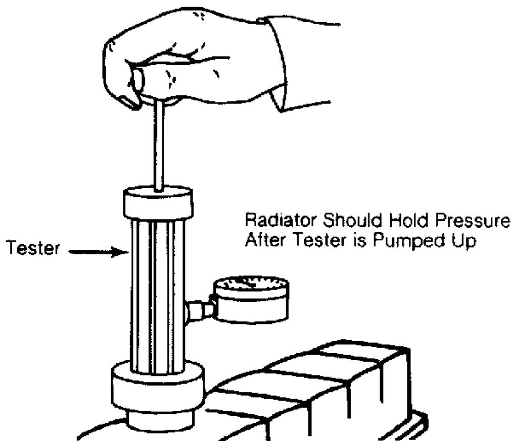
Fig. 3: Pressure Testing Cooling System
