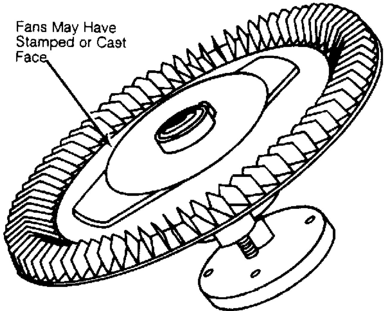
Fig. 7: Thermostatically Controlled Fan Assembly
