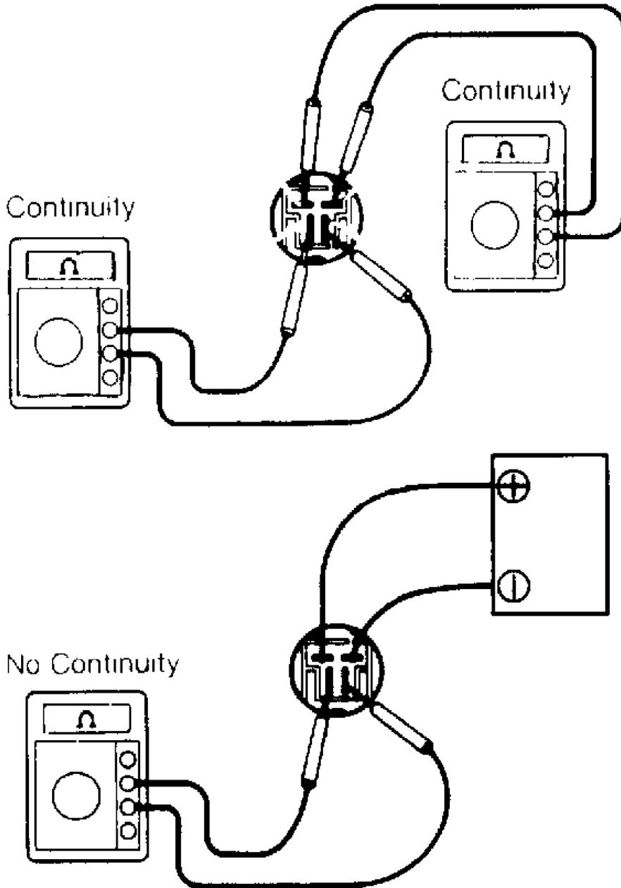
Fig. 8: Testing Cooling Fan Relay
