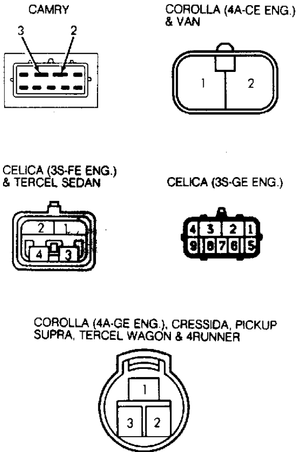
Fig. 11: Neutral/Start Switch Connector Terminal Identification Courtesy of Toyota Motor Sales, U.S.A., Inc.
