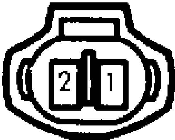
Fig. 14: Speed Sensor Connector Terminal Identification (CELICA) Courtesy of Toyota Motor Sales, U.S.A., Inc.
