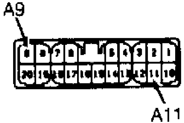
Fig. 13: Speed Sensor Connector Terminal Identification (CAMRY) Courtesy of Toyota Motor Sales, U.S.A., Inc.
