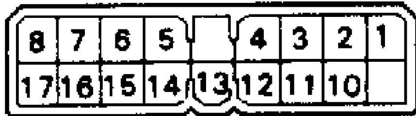
Fig. 6: Computer Connector Terminal Identification Courtesy of Toyota Motor Sales, U.S.A., Inc.
