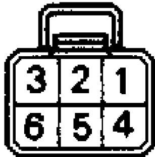
Fig. 21: Actuator Terminal Identification Courtesy of Toyota Motor Sales, U.S.A., Inc.
