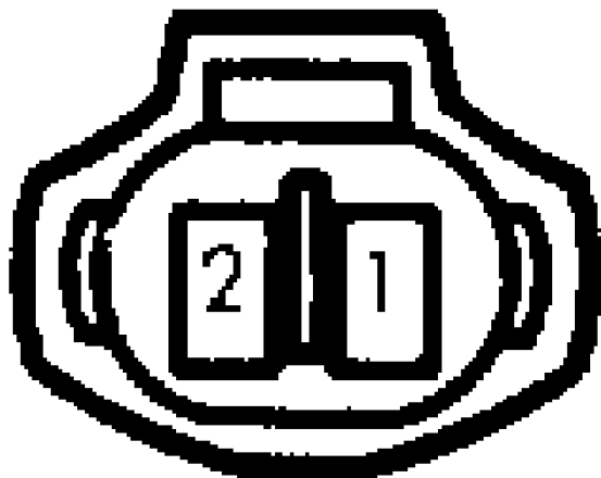
Fig. 10: Speed Sensor Connector Terminal Identification Courtesy of Toyota Motor Sales, U.S.A., Inc.
