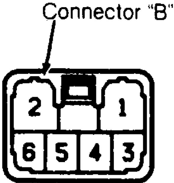
Fig. 4: A/C Switch Terminal Identification (Push Button Type)
