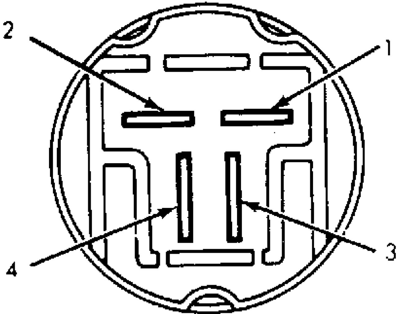
Fig. 5: Checking Radiator Fan Relay
