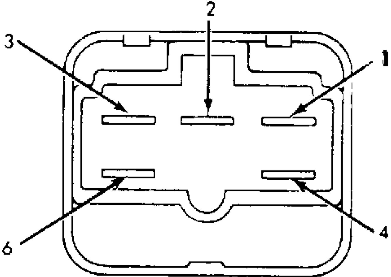
Fig. 6: Checking Condenser Fan Relay No. 2
