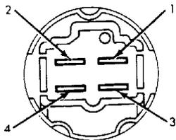
Fig. 7: Checking Condenser Fan Relay No. 3
