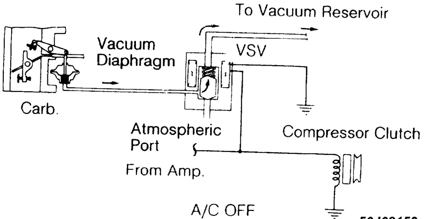
Fig. 1: Schematic of Vacuum Switching Valve (A/C Off)
