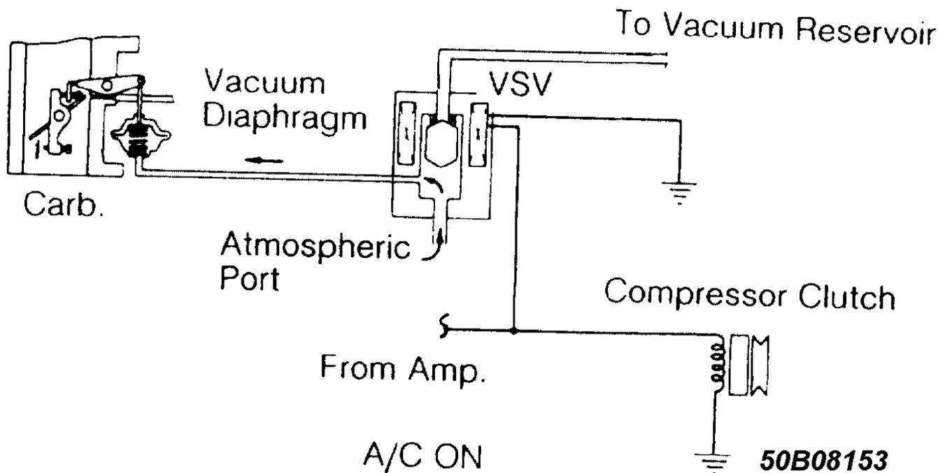
Fig. 2: Schematic of Vacuum Switching Valve (A/C On)
