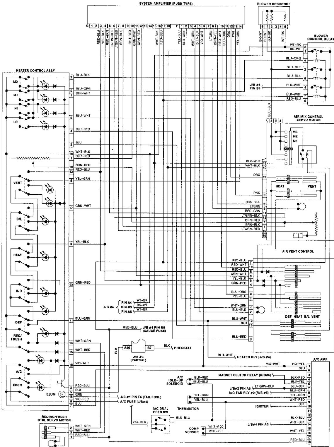
Fig. 13: Push Button System Wiring Diagram (1 of 2)
